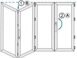
③ Slide first pair of panels together and continue moving folded pairs to end.
