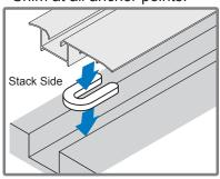
Slide Guide along Sill to test. Adjust screws to level track.
