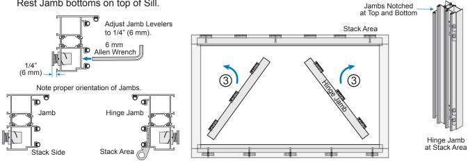
(3) Measure opening at top, middle, and bottom and compare to opening measurement on Shop Drawings. Adjust Levelers as needed.
