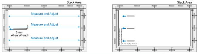
NOTE: Final lateral adjustments may be required after panels are installed.
