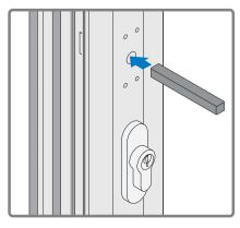
Install Handles on each side with included screws.
