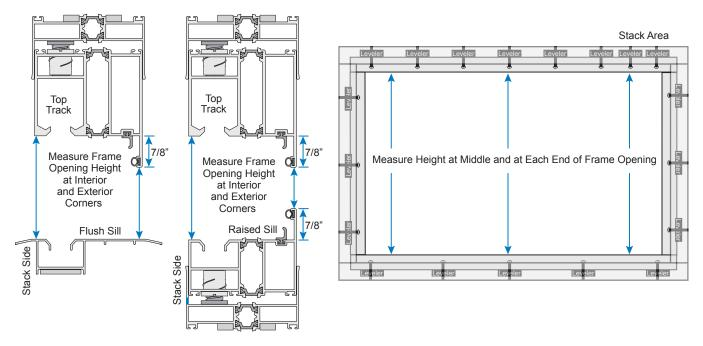
(2) Measure from top to bottom of each Door Frame excluding the gasket.
