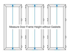
③ Check both measurements against Shop Drawings. Calculate clearance to ensure proper door operation.
