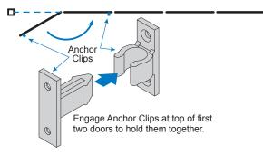
(3) Fold third door away from track and slide with first two doors. Repeat until all doors are folded together at one end.
