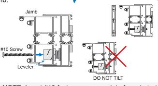
NOTE: Insert #10 fasteners appropriate for substrate into center of Levelers to secure. Do not overtighten fasteners.
