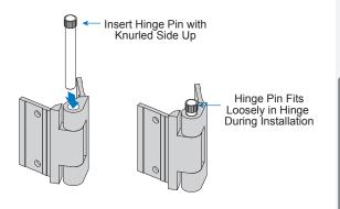
NOTE: Use included C-Clamps to secure Hinge Pins after all door panels are installed. Do not ever hammer or force pins into place as this will damage the doors. Do not secure until installation is complete.
