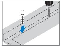
Secure but do not over tighten. Shim to prevent movement.
