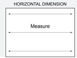
Measure side to side at top, middle and bottom to confirm proper width.
