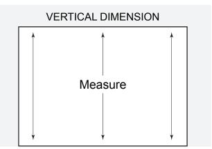
Measure top to bottom at left, center, and right to confirm proper height.
