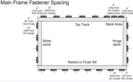
IMPORTANT: Levelers are factory installed at Jambs, Head and Sill. Fasten at each Leveler location with #10 fasteners appropriate to carry load. Fastener Heads larger than 1/2" (13 mm) wide by 3/16" (5 mm) tall can damage Rollers. Do not overtighten fasteners. This can damage frame and interfere with door operation.
