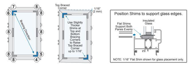
NOTE: When installed, the doors pull down slightly due to weight and the out of square doors become almost even. If there are any issues with door operation, shim thickness needs to be adjusted. Doors must be braced correctly for proper operation.
