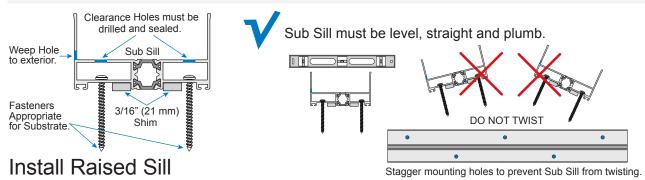
IMPORTANT: Do not overtighten fasteners. This can cause frame to bow and/or distort and interfere with door operation. Ensure Sill is flat and level and does not tilt inward or outward. Clean cuttings from drill holes and any other debris from track.
