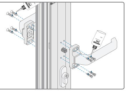
\* Loctite<sup>®</sup> is recommended on all screw threads during final assembly.
