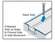
Drill holes 3" (76 mm) from ends and 20" (508 mm) on center.
