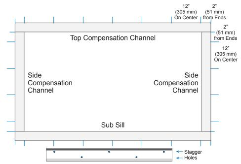
IMPORTANT: Use fasteners appropriate for substrate. Stagger fastener holes to prevent Compensation Channel and Sub Sill from twisting.
