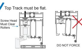
(6) Lower Top Track so it rests on Jambs. Level and secure with fasteners appropriate to carry the load.
