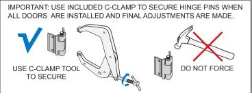
Insert 4-1/2" Hinge Pin with Knurled Side Up
