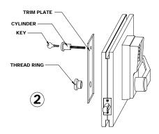
REMOVE CYLINDER BY INSERTING KEY AND ROTATING CYLINDER ANTI-CLOCKWISE UNTIL IT IS FREE.
