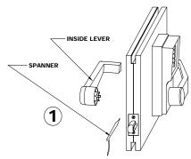
REMOVE INSIDE LEVER BY INSERTING POINT OF SPANNER INTO POKEHOLE IN COLLAR OF DRIVE SLEEVE AND DEPRESSING RETAINING CLIP.
