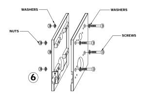
SEPARATE CLAMP PLATES BY REMOVING 4 CAP HEAD SCREWS NUTS AND WASHERS.
