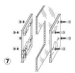
ASSEMBLE CLAMP PLATES ONTO GLASS.
