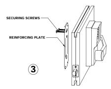
REMOVE REINFORCING PLATE BY UNSCREWING THE TWO SECURING SCREWS
