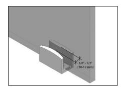
6. Install Floor Guide(s) just beyond the edge of the opening or center of the overlap. The Floor Guide must be adjusted to fit your glass thickness prior to securing it to the floor. Mark the centerline of door panel(s) and the Guide(s) on the floor.
