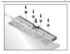
1. For 3/8" (10 mm) Glass, insert Spacer Pins and Regulator Bolt Nut with short ends up. Position Clamp Assembly along the top edge of the glass, a minimum of 1-3/4" (45 mm) from the vertical edge.
