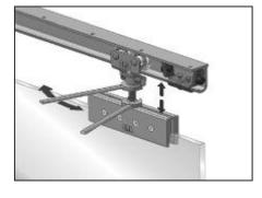
8. Adjust Door Panel to be plumb with jamb and to desired floor clearance by turning the Upper Adjusting Nut counterclockwise to lower the panel and clockwise to raise the panel.
