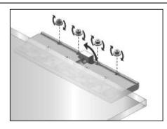
2. For 1/2" (12 mm) Glass, insert Spacer Pins and Regulator Bolt Nut with tall ends up. Position Clamp Assembly along the top edge of the glass, a minimum of 1-3/4" (45 mm) from the vertical edge.
