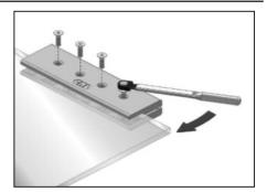
3. Attach second half of clamp with supplied flat head Allen screws. Tighten to recommended torque of 11 lbs./ft. (15 Nm). Repeat steps 1-3 for second Clamp Assembly.
