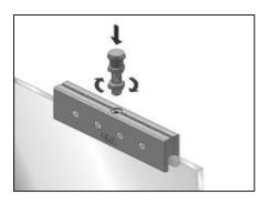
4. Screw in Regulator Bolts until they bottom out. This will allow for maximum clearance at the bottom of door, and makes hanging the door panel easy. Door alignment and clearance adjustments are shown later in Step 8.
