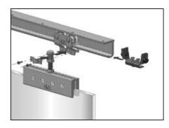
5. Hang Top Track plumb and level using appropriate fasteners (not included). Insert Rollers and Stops into Track. Attach Regulator Bolts to Rollers using Regulator Bolt Strap and Fasteners supplied with each Roller.
