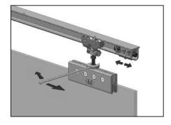
9. Secure adjusted panel by tightening the Lower Adjusting Nut against the clamp assembly. Adjust Roller Stops and secure.
