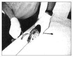
**11.\*** *HEADLINER WRAP OPTION:* The use of an electric shear is recommended. **Do not** cut through the headliner. The use of a sabre saw will require lowering or removing the headliner.
