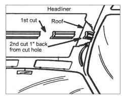
**12.** Remove any debris from the roof. Trim back roof bows so that they are no closer than 1" from the cut edge of the sunroof opening. The cut end of the bow should be flattened and secured to avoid rattles and sharp points. If necessary, reconnect and/or relocate any wiring. Secure wiring, at least 2" beyond the cut hole, to prevent rattles.
