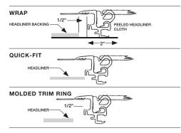
**15.\*** *WRAP HEADLINER INSTALLATION*: Cut out the headliner 2" smaller than the roof cut opening. Carefully peel the cloth headliner material from the hardboard backing to a line 1/2" larger than the roof cut opening. Cut and remove the excess hardboard material back to the 1/2' line. Caution: Do not cut into the cloth material.
