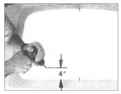
**10.** Drill a pilot hole 4" inside the cut line. The pilot hole size will be determined by your choice of cutting tool. **It is important not to damage the headliner.**
