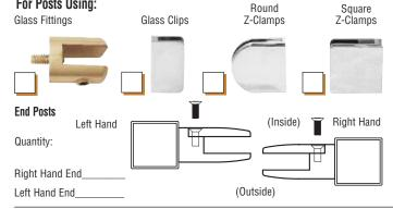
Glass is held in place with Clips, Clamps or Fittings mounted to the Partition Posts. Diagrams below give you the option for placement of exposed screw heads.
