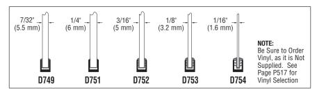
CRL Design Series Partition Posts come with 5/16" (8 mm) U-Channel which can be used to glaze five different thicknesses of materials.
