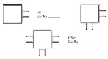
Glass is held in place by U-Channel mounted to the Partition Posts.
