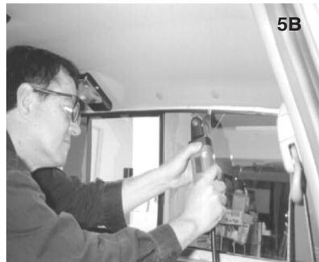
Using CRL Wildcat Urethane Cut-out Knife and CLR Wildcat Blade, cut out backglass from inside the truck cab. Place a protective cover over the truck bed, and cover the seat with a plastic sheet. See photos 5A and 5B and diagram 5C.
