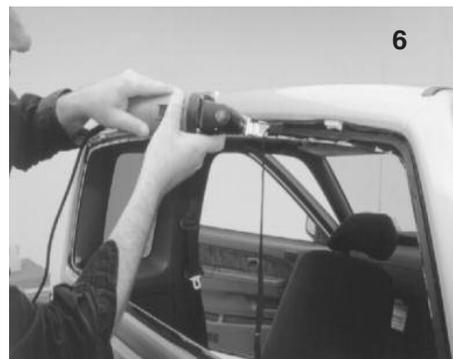
Using CRL Chisel Blade, trim down existing urethane bead all the way around opening. See photo 6.
