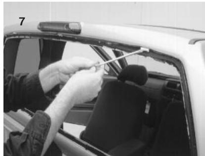
Place the the Tri-Vent into cab opening and check for a flush fit. Any adjustment to window fit or curvature should be made before sealant is applied. See photo 8. Note the light on the outside cab above the rear window opening. If it interferes with installation, remove it and put it aside.
