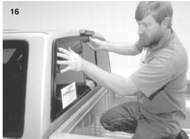
While your helper pushes on the Tri-Vent frame from the outside, use a slotted screwdriver to push the clips into place over the pinchweld lip. See photo 18. These tabs secure the Tri-Vent while the sealant cures, and allow the truck to be driven immediately after installation.
