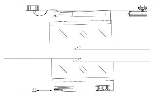
Check alignment of with Head and Jamb. If adjustment is required, follow procedures in Rail Assembly Instructions. When Leaf is aligned correctly, re-install End Caps.
