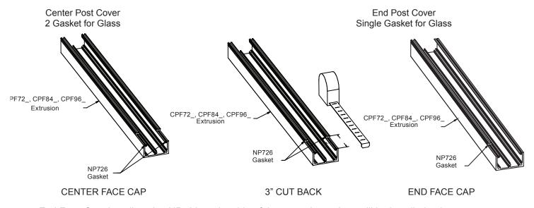
End Face Cap: Install gasket NP726 on the side of the post where glass will be installed only.
