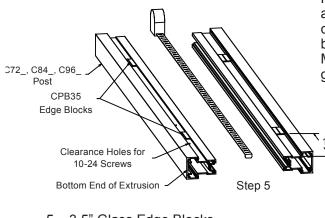
5. 3.5" Glass Edge Blocks installation: Peel adhesive back and place (2) edge blocks alongside glazing channels, 15" from each end.
