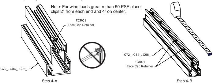
Align and insert snap clip's tabs into center channel. Turn clockwise \( \frac{1}{4} \) to lock in place. DO NOT USE SCREWDRIVER TO INSTALL CLIPS. Pliers may be used to make the ¼ turn.
