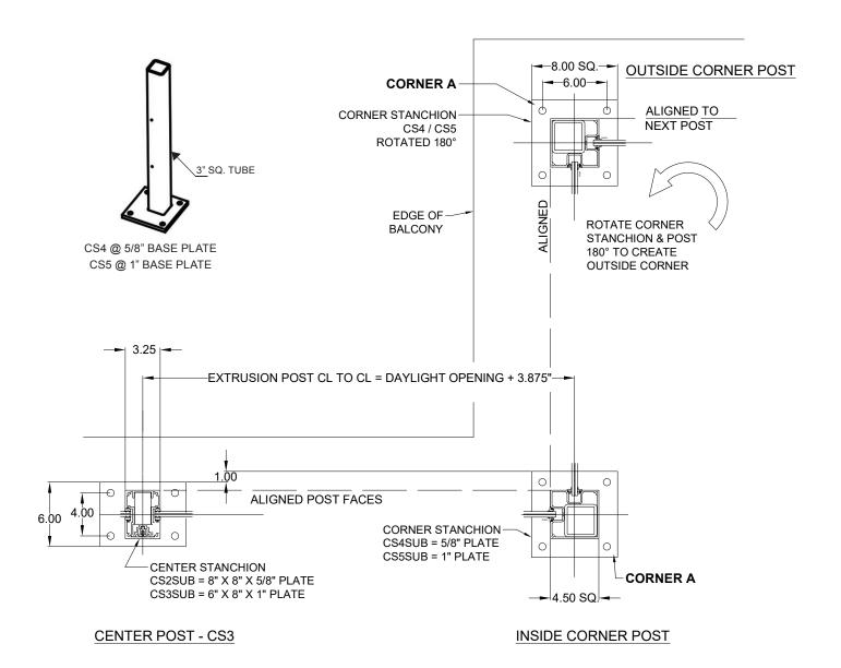
CORNER POST STANCHION LAYOUT- TEMPORARILY PLACE ALUMINUM EXTRUSION OVER STANCHION TO ALIGN GLASS POCKET CENTER LINES, AS SHOWN IN DIAGRAM. ALUMINUM POST AND STANCHIONS MUST ALWAYS BE ASSEMBLED IN THE SAME ORIENTATION TO EACH OTHER. ROTATE STANCHION AND POST TO ACHIEVE DESIRED RAILING CONFIGURATION. POSITION OF STANCHION AND ANCHORING HARDWARE MUST SPECIFIED BY STRUCTURAL ENGINEER.
