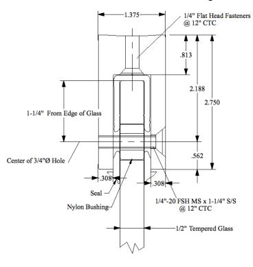
Tension connection between the legs from the through screw is required for the base shoe to support the maximum moment:
