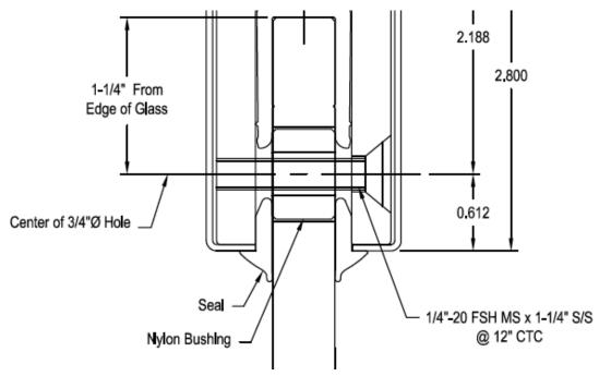
Screw shear strength - 1/4" Countersunk stainless steel flat head screw, Alloy group 1, condition AF, ASTM F593 equivalent.
