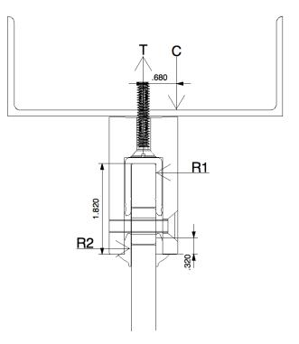
Base shoe strength won't determine allowable load or light size for any of the glass thicknesses or types that may be used with the B5B shoe.
