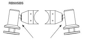
Swivel Fitting Designed for segment applications. Each Swivel Fitting is adjustable up to 8 degrees.
