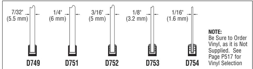
CRL Design Series Partition Posts come with 5/16" (8 mm) U-Channel which can be used to glaze five different thicknesses of materials.
